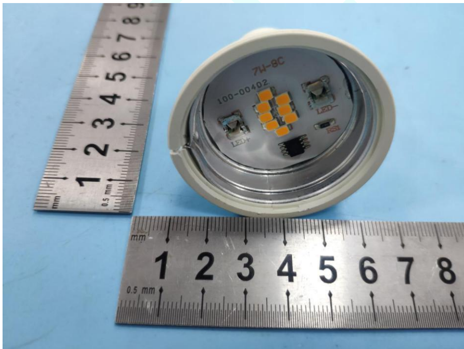
Photo 6 - LED module of CT- 4216
